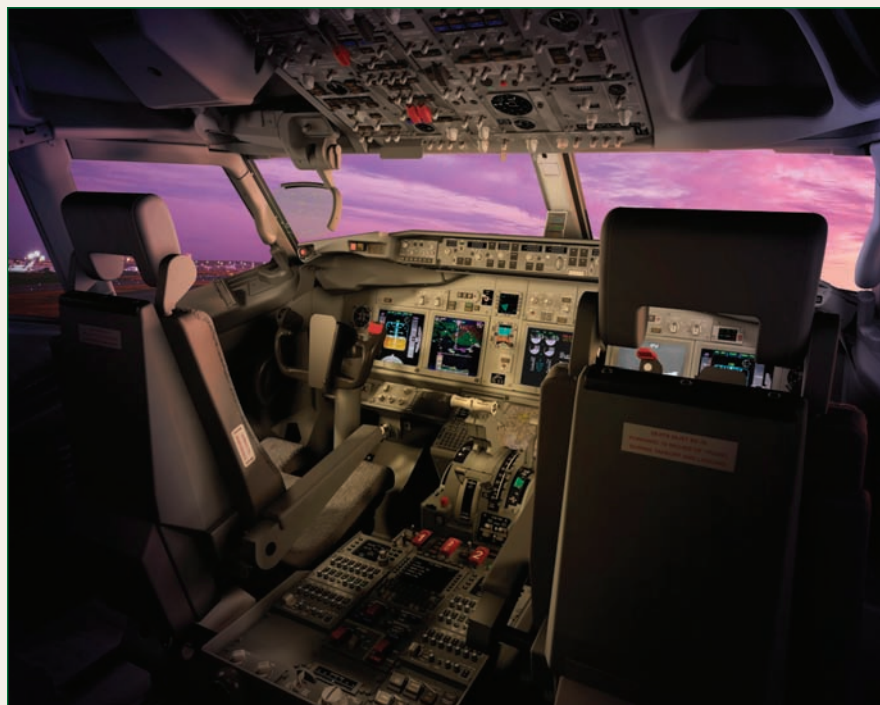
Figure 1 | The P-8A Poseidon cockpit uses test display panels from Parvus Corporation to track the operation of various electrical components inside the aircraft. (Photo courtesy of Boeing.)
